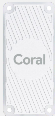
TPU Google Coral Google Edge TPU ML accelerator coprocessor
