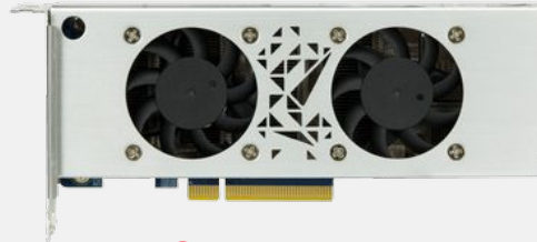
FPGA Intel Arria 10 IEI Mustang-F100-A10
