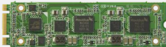
VPU Intel Myriad X (x2) UP AI Core XM 2280 (M.2)
